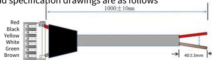
Schematic diagram of control line cable arrangement and specifications
